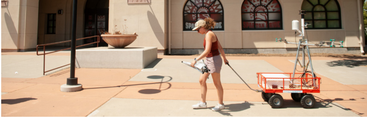
A CivicSpark Fellow prepares a mobile biometeorological instrument for data collection at a school bus stop. Credit: Sacramento Metropolitan Air Quality Management District.
